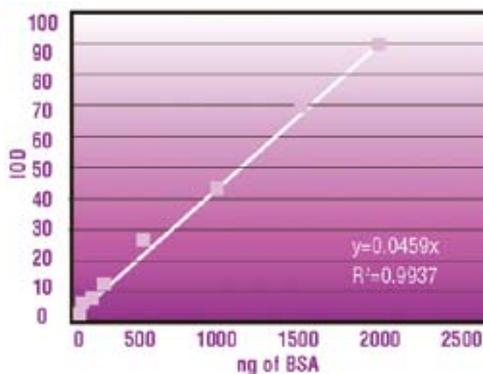
Band intensity was measured and plotted against the amount of protein (BSA) loaded per gel lane. The result shows a linear dynamic range from 5ng to 2000ng using EZ-Run Protein Gel Staining Solution.
